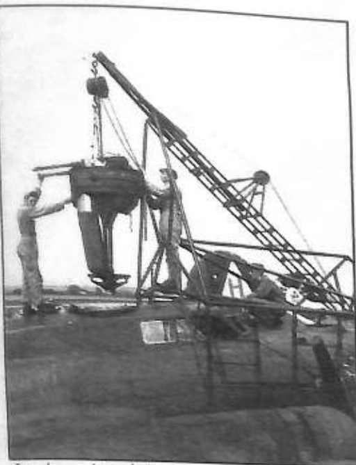
It takes quite a hoist to get a top turret back in its "home."
